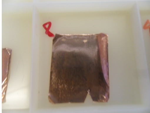
Figure S1. Copper foil with CVD graphene grown following the methods from section I.
