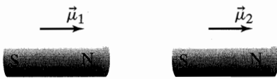
Figure 21.50 The magnetic dipole moment \mu_2 of the second magnet lies along the axis of \mu_1 of the first magnet.
