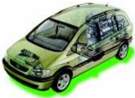
The Opel Zafira, by General Motors, reforms methanol to operate a polymer electrolyte membrane fuel cell. This vehicle has nearly zero emissions of sulfur dioxide and nitrogen oxides and the carbon dioxide output is expected to be 50% less than a comparable internal combustion engine vehicle. (Courtesy: General Motors)
