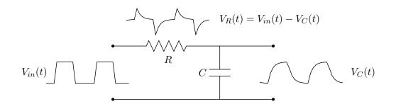
The CR circuit is easy to analyze in the time-domain, again because  $V_{\circ}(t) = V_R(t) + V_C(t)$ . The picture below shows the waveforms resulting from the time-domain analysis which we have already performed. The CR circuit acts as a differentiator of an input waveform over times small compared to  $\tau$ .
