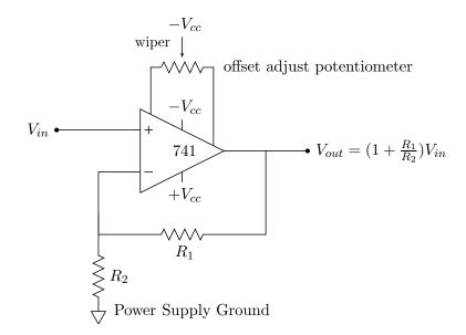
If this correction is not performed, the constant offset potential  $V_o$  will produce a constant background,
