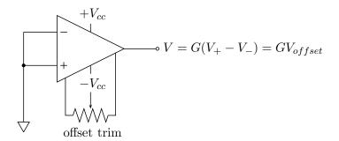
If  $V_{offset}$  is bothersome, one must ground the inputs of whatever amplifier has been built and adjust the offset-nulling trimpot. For example, in the noninverting configuration,  $V_{in}$  must be grounded and the trimpot adjusted to zero the output.
