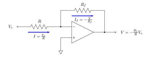
Using the facts that  $I = I_f$  and  $V_- = V_+ = 0$ ,
