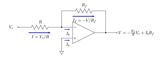
The analysis is based upon conservation of current,  $I = I_b + I_f$ , and the fact that  $V_- = V_+$ :
