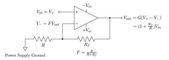
The relationship between the input and output signals for this *noninverting amplifier* configuration is
