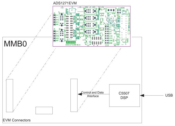
Figure 2. ADS1271EVM-PDK Block Diagram
