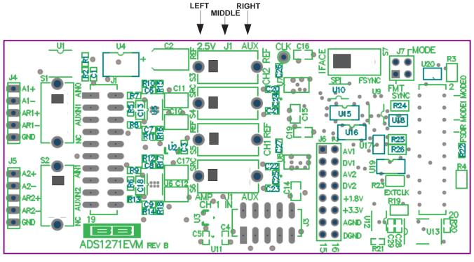
Figure 1. ADS1271EVM Switch and Jumper Locations
