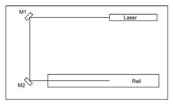
The U geometry is defined by the two mirrors labeled M1 and M2 in the diagram. The goal of this experiment is to ensure that the laser beam (i.e. the optical axis) is parallel to the table top and aligned above the center of the rail. Mount M2 on the optical table and position it close to the beginning of the optical rail such that the center of the mirror is above the center line
