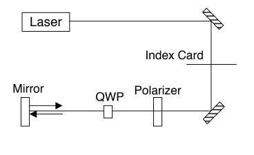
A quarter-wave plate is designed so that the fast and slow components of a wave will experience a relative phase shift of  $\pi/2$  (1/4 of  $2\pi$ ) upon traversing the plate. Light that enters the plate linearly polarized at 45° with respect to the fast and slow axes will then leave the plate circularly polarized.
