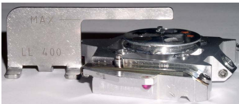
FIGURE 5-21 SETTING OF SAMPLE HEIGHT
