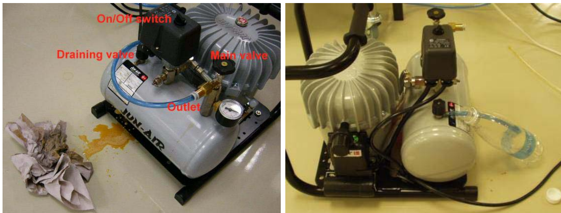
FIGURE 6-2 COMPRESSOR CONDENSATE DRAINING
