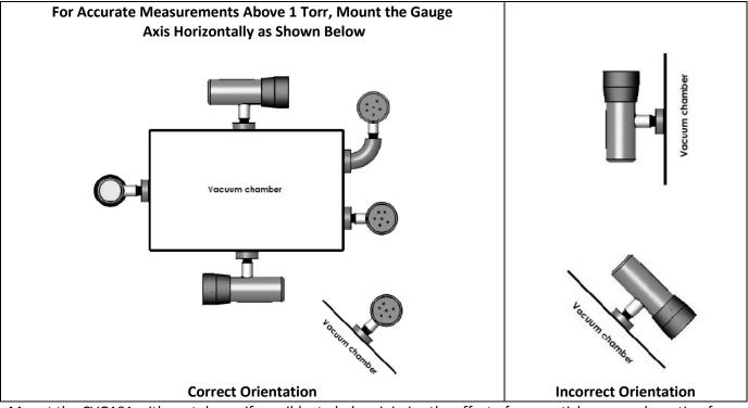
Mount the CVG101 with port down, if possible, to help minimize the effect of any particles or condensation from collecting in the gauge.
