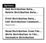
**Normalize distribution** is a command that scales the distribution data so that the maximum intensity of the distribution is 100%.
