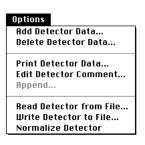
**Normalize Detector** is a command that scales the detector data so that the maximum efficiency of the detector is 100%.
