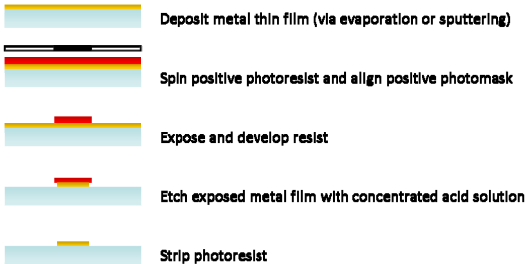
Figure 3.2: Wet etching schematic process flow. The sky blue rectangle represents the substrate, while the yellow and red materials symbolize the deposited film and photoresist, respectively. Note: dimensions not to scale.
